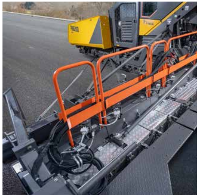
Hose and cable routing channel
